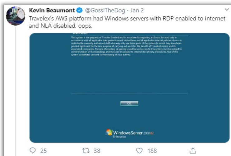
Figure 13 - Exposed Traveler Windows Server with RDP enabled/NLA disabled
