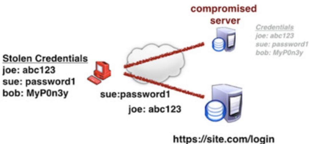
Figure 3: Credential Stuffing attack diagram by OWASP.<sup>3</sup>
